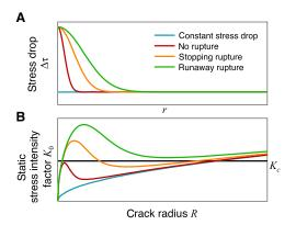
**Fig. 5. Fracture mechanics of rupture arrest under nonuniform stress.** Sketch of **(A)** stress drop distributions  $\Delta \tau(r)$  and **(B)** the corresponding static stress intensity factors  $K_0(R)$  illustrating different crack behavior (although our approach supports  $K_c$  being a function of R, for illustration purposes,  $K_c$  is plotted as a constant).
