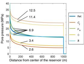
Fig. 3. Comparison of pore-pressure distribution inside sealed cylindrical reservoirs induced at time t = 100 days by steady-flux injection at its center, for varying compressibility  $c_{tr}$  viscosity  $\mu_{vr}$ , porosity  $\phi$ , and permeability k. Higher and lower values of parameters are depicted by thicker and thinner lines of the same color, respectively. The numbers indicate the values of the spatial integral of pressure in megapascals per square kilometer.
